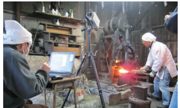
Inspection of the process of Japanese sword production using infrared thermography
