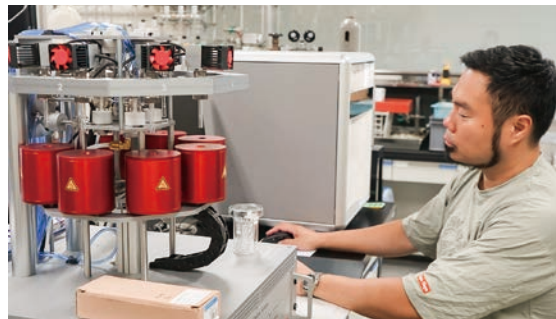
Automated graphitization equipment for radiocarbon dating (REKIHAKU)
