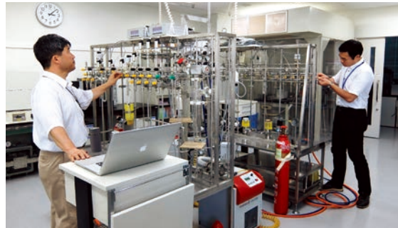
Vacuum line to prepare sample for radiocarbon dating (Rekihaku)
